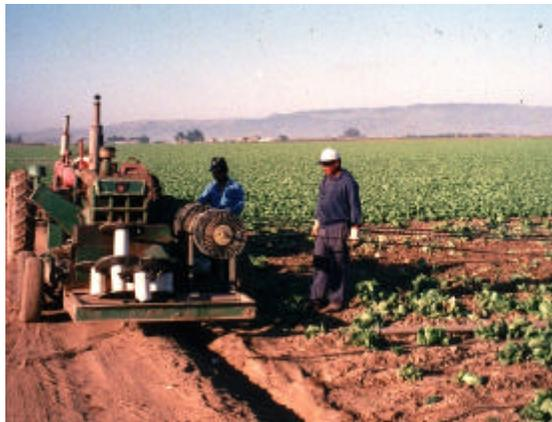
Figure 10. Example of a homemade retrieval trailer, powered by an old tractor engine.
