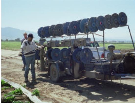
Figure 9. Commercially available tape extraction machine.
