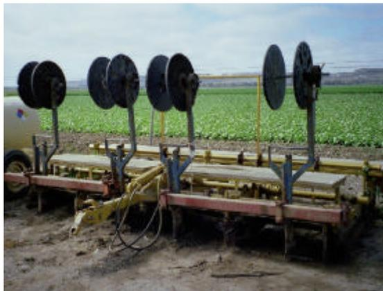
Figure 4. Three point hitch commercially available injection system.
