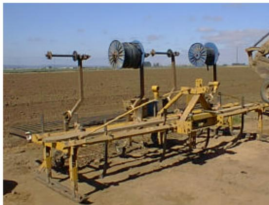
Figure 6. Homemade injector heads.
